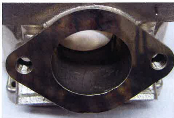
■ The top edge of the exhaust port may show either just a cast finish surface:
