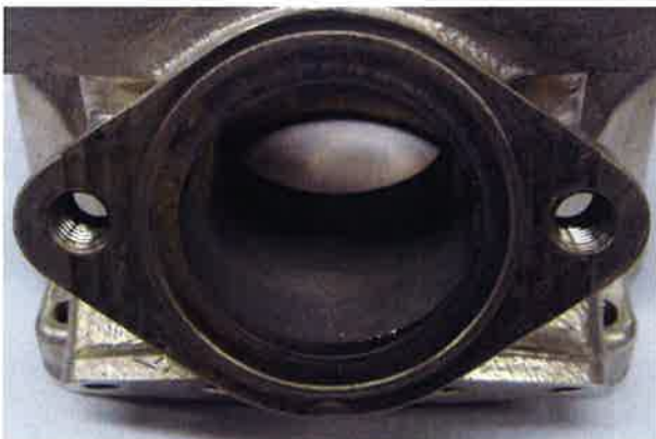
■ The flange for the exhaust socket may show either cast finish or machined surface. Machined surface can be either flat or show a circular sealing bump.
