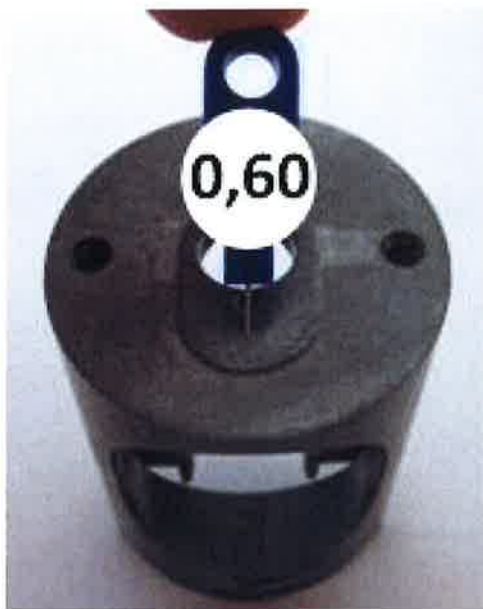
17.10.15) Vertical bore of carburettor insert Plug gauge 1,30 may not enter the bore (use jet gauge set Rotax part no. 281 920).
