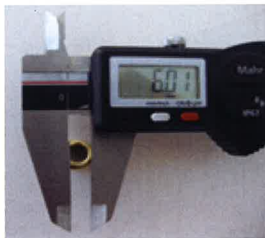
17.10.12) Atomizer, dimension of cross bore: 5,0 +/- 0,15 mm
