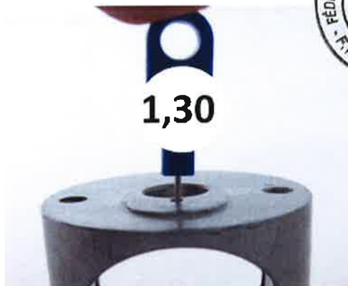
17.10.15) Vertical bore of carburettor insert Plug gauge 1,30 may not enter the bore (use jet gauge set Rotax part no. 281 920).
