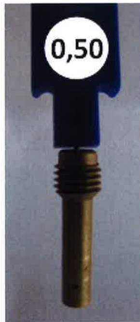
17.10.8) Idle emulsion tube Idle emulsion tube has to be stamped with 45. Plug gauge 0,50 may not enter the central bore. (use jet gauge set Rotax part no. 281 920)
