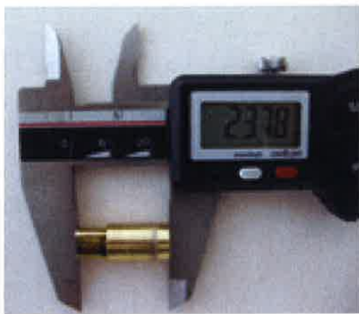
17.10.10) Atomizer, length of cylindrical part: 15,75 +/- 0,25 mm
