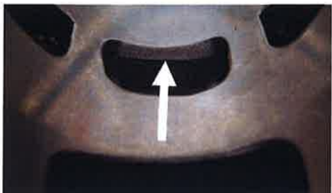
■ The upper edge of the central boost port may show factory machining.
