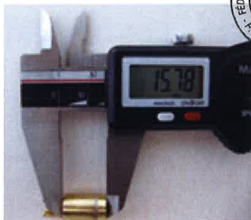
17.10.10) Atomizer, length of cylindrical part: 15,75 +/- 0,25 mm
