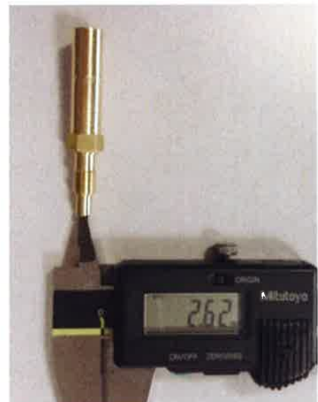
17.10.7) Idle jet Idle jet has to be stamped with 60. Plug gauge 0,65 mm may not enter the bore (use jet gauge set Rotax part no. 281 920).
