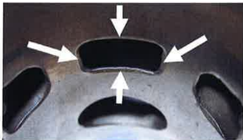
■ The upper edge of the central boost port may show factory machining.
